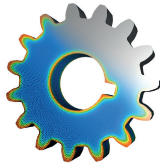
Surface heat treatment (carburizing, quenching, tempering)
