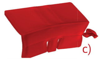
Observation after computing part deformation: a) Adaptive automatic remeshing b) Projected deformation c) Deformation amplified x10
